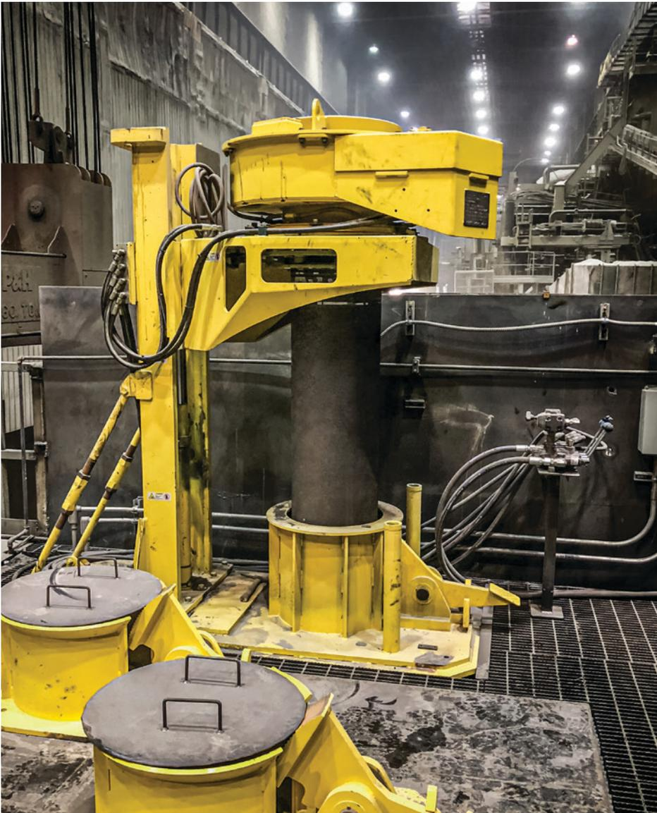
**SPINNING HYDRAULIC TORQUE DEVICE**
